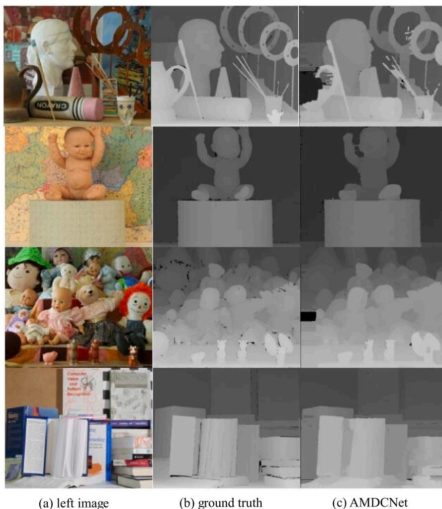
**Fig. 10.** Performance evaluation using Middlebury test data. (a) left image of stereo image pair, (b) ground truth disparity, and (c) disparity map estimated using AMDCNet. Top to bottom: four types of images are art, baby, dolls and book.
